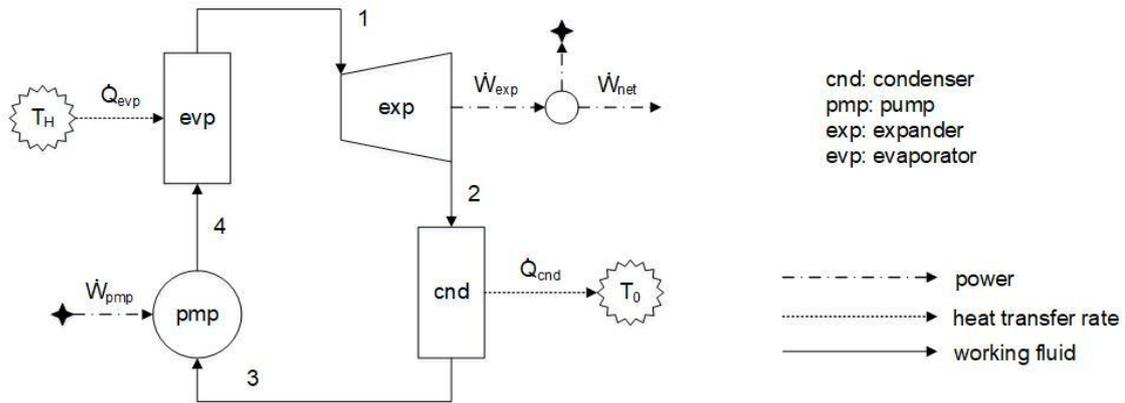
Figure 2: Productive diagram of the ORC
