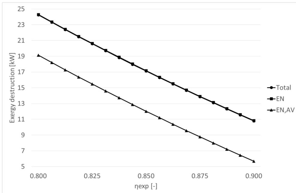
Figure 6: Results from the parametric analysis of the pump
